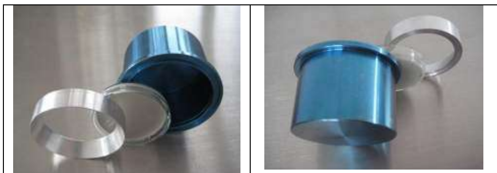
Figure 26 Outgassing test – cover ring
